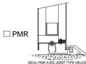
**PORTE BATTANTE UN VANTAIL COUPE FEU EI 120 REF: NT EI120.1 POSE APPLIQUE BETON**
